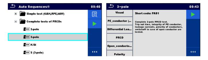
The combination of the different functions are built into several AUTO SEQUENCE®s which guide the user through complete and professional testing of P-RCD protected extension leads or portable switchgears. This functionality makes MI 3360 OmegaPAT XA a leading tester in this application. With the provided information the user can easily identify if the equipment has some malfunction. One of the typical problems could be faulty power supply capacitors.
